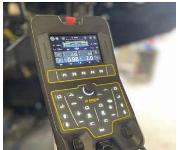
Screen side panel with large full graphic display - direct access to all major functions
