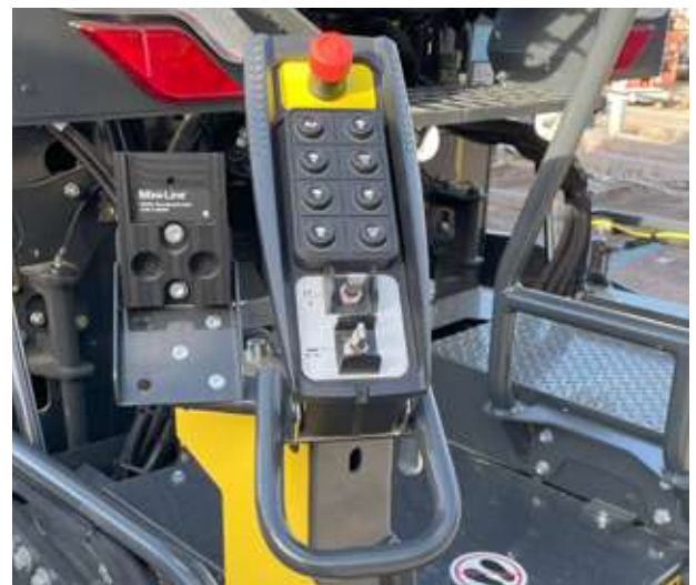
EASY-PAVE - simplified and intuitive side control panel concept
